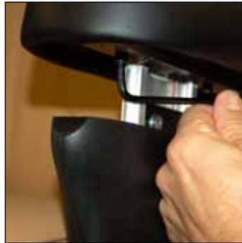
2. With both shroud screws loose, push the shroud down for open access to the 3/16" Allen-head bolts that secure the arm pad to the post, and then remove both.
