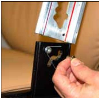
5. Reverse steps to replace aluminum "T" and pin and spring. Make sure the "T" is properly engaging click-stops as you lift it, and as the other armrest works.
