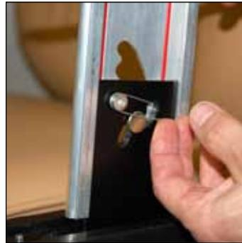
3. Remove the aluminum "T" by first disassembling the spring assembly (take notice of steps as you will reverse them shortly). Lift both ends of the silver spring out of the slot, and then lift up on "T" until you find position allowing removal of the brass pin. Remove pin, and slide "T" up and off.
